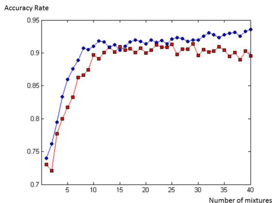
**Fig. 2.** GMMs accuracy rate evolution when increasing the number of Gaussians using the original feature vector (in red) and using the feature vector populated with the time-coefficients (in blue).
