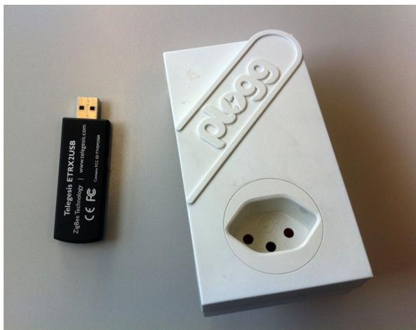
**Fig. 1.** A PLOGG acquisition device and the communication ZigBee USB dongle
