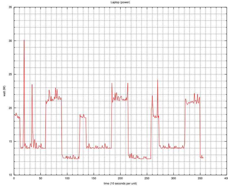
Fig. 2. Example of the active power consumption measured on a laptop
